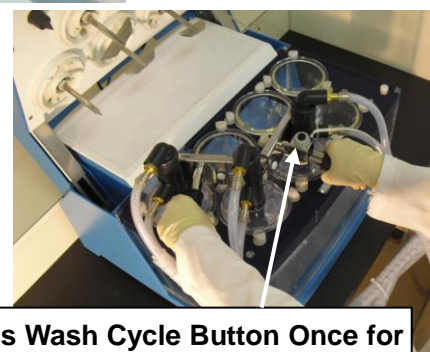
2. Turn on Main Switch to Evacuate Spent Media
