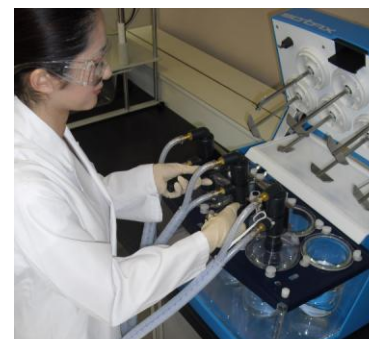
2. Turn on Main Switch to Evacuate Spent Media
